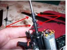
The lower rotor head is affixed to the outer drive shaft by four screws. As with the retaining collar step, back the screws all the way out, then screw them back in slightly to prevent loss of the screws. Replacement lower rotor heads do not currently come with new screws.
