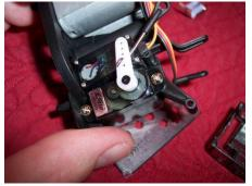
The port side servo is held by two screws.
