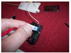
To disassemble the 4in1, so that you can ventilate the case without damaging the electronics, first remove the RX crystal.
