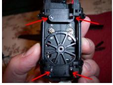
Remove the four screws that hold the battery tray to the main frame.
