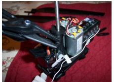
Gently remove the linkages from the swashplate's ball joints. This can be done with your fingers, however ball link pliers will make this task easier and reduce the likelihood of inadvertent damage to the links and ball joints.
