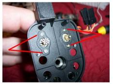
Each of the rotor motors are held in place by two screws through the main frame. Removal of these screws will allow for the removal of the drive motors.
