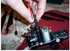
Once all four screws have been sufficiently loosened, gently pull the lower rotor shaft from the outer drive shaft.
