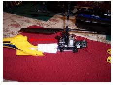
Gently slide tail section off of frame and antenna.
