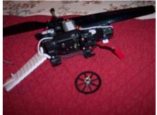
The drive gear and collar can then be removed, as it will be loose in the battery bracket.
