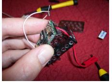
By pushing gently on the battery lead, and pulling gently on the circuit board, the adhesive that holds the board inside the case should break free and allow removal of the 4in1 board from its case.
