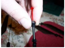
Gently pull the cap at the end of the outer drive shaft that holds the bearing for the inner drive shaft.
