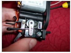
The starboard side servo is held by one screw at the top and double stick tape at the bottom.
