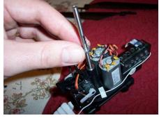
Slide the retaining collar up and off of the outer drive shaft.
