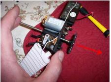
The outer rotor shaft will now be free to be pushed fully out of the main frame.
