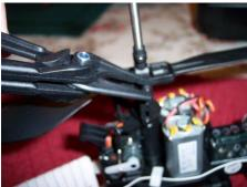
Gently remove the linkages from the lower blade's ball joints. This can be done with your fingers, however ball link pliers will make this task easier and reduce the likelihood of inadvertent damage to the links and ball joints.
