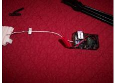
Set the 4in1 and antenna aside. This would be a good time to ventilate the plastic case of your 4in1 to reduce tail drift.
