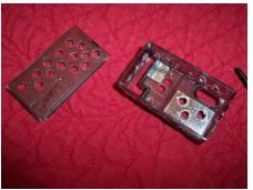
The empty case can now be safely cut or drilled to perform a 4in1 cooling mod.
