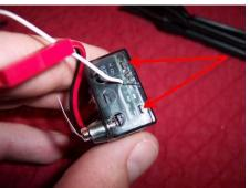
Use a precision flathead screwdriver to gently push the two small retaining tabs on the opposite end of the 4in1 case.
