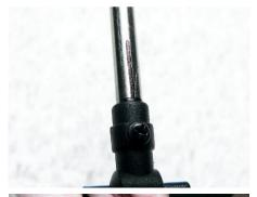
This photo, and the one that precedes, were posted by LRHann. He recommends to mark the outer drive shaft with a sharpie horizontally at the top of the rotor hub, and vertically in line with the set holes. This makes lining up the screws easier during reassembly.
