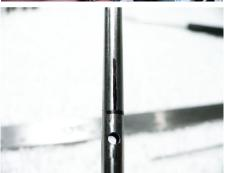
As a note for reassembly, the upper screws of the rotor head must align and set into the holes of the outer drive shaft.
