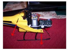
Remove the canopy and slide the two CF rods out of the frame and tail section.
