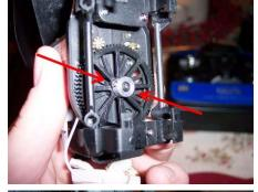
To remove the drive gear for the inner shaft, loosen the screws on each side of the aluminum retaining collar. This will allow the inner shaft to be pulled out of the rotor mast.
